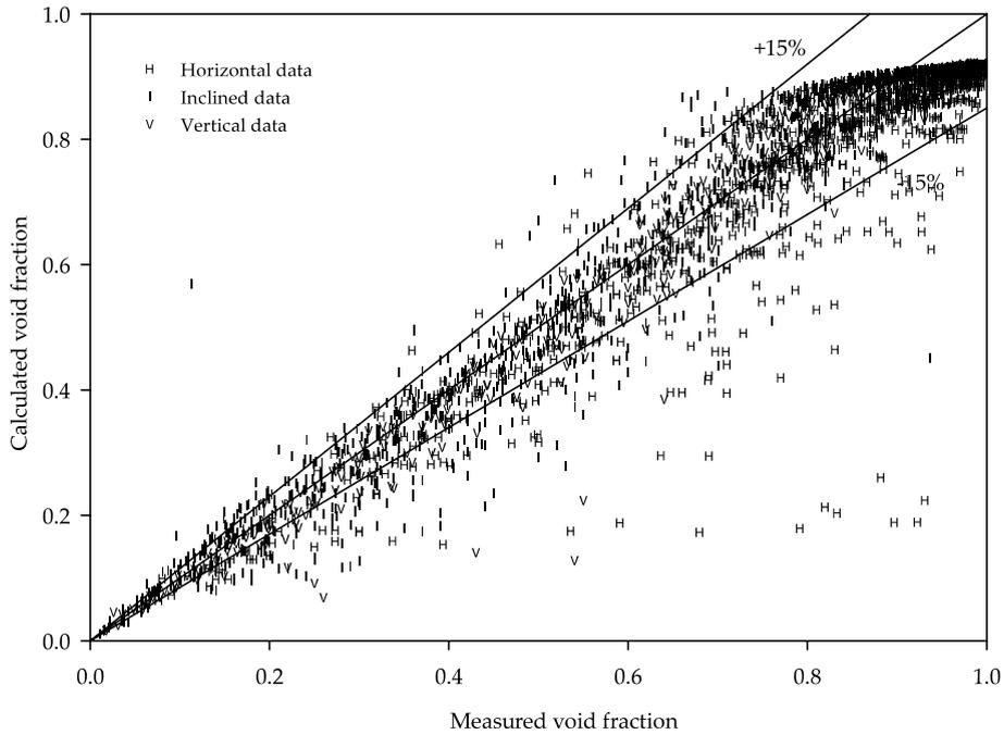
Fig. 4. Comparison of Toshiba (Coddington and Macian, 2002) correlation with measured combined total experimental data.
