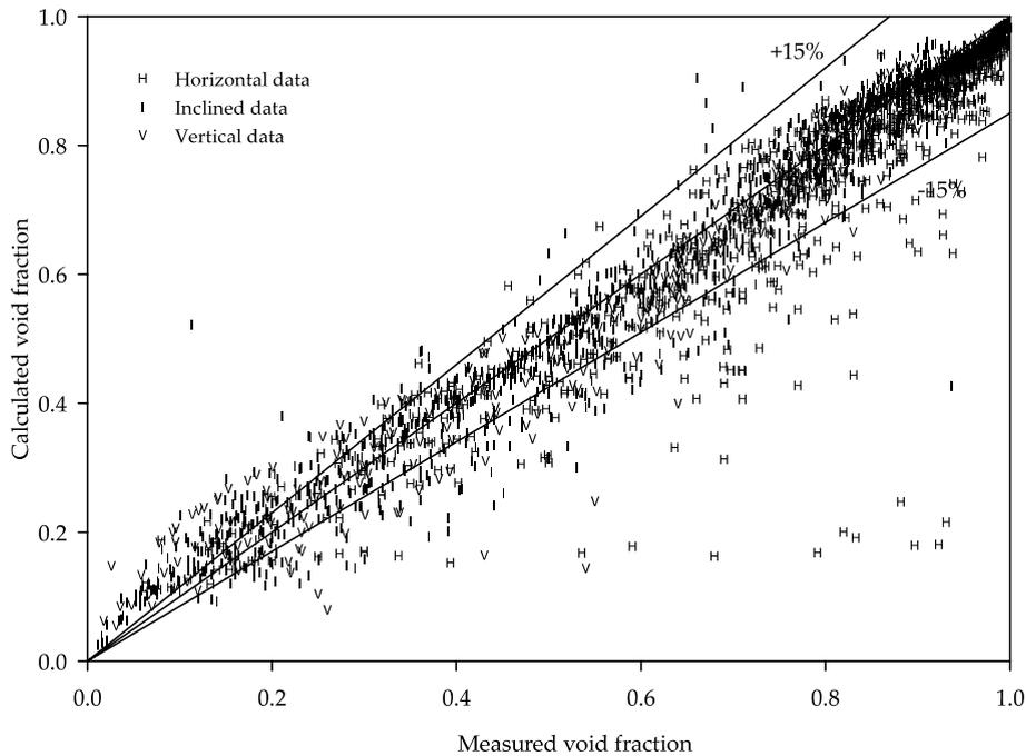
Fig. 6. Comparison of Dix (Coddington and Macian, 2002) correlation with measured combined total experimental data.
