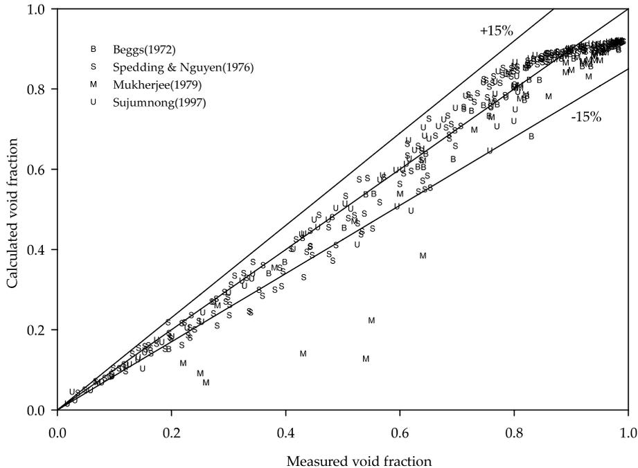
Fig. 3. Comparison of Toshiba (Coddington and Macian, 2002) correlation with measured combined vertical experimental data.
