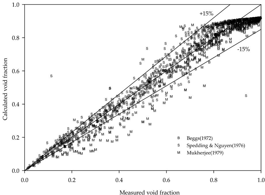
Fig. 2. Comparison of Toshiba (Coddington and Macian, 2002) correlation with measured combined inclined experimental data.
