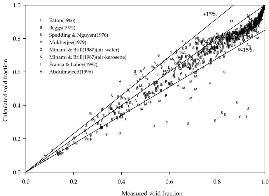
Fig. 1. Comparison of Rouhani I (1970) correlation with measured horizontal experimental data.
