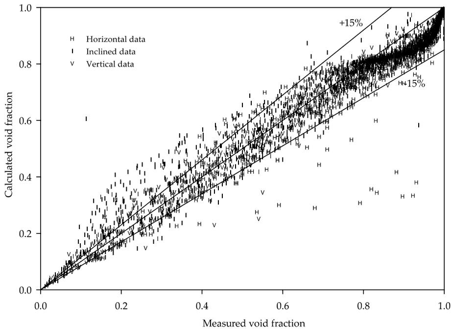
Fig. 5. Comparison of Rouhani I (1970) correlation with measured combined total experimental data.
